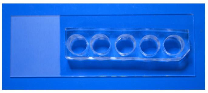
Fig 1. Picture of the homemade PDMS chambers for liposome production. The chamber size is 8 mm in diameter and 10mm in height). PDMS firmly adheres on a glass slide.
