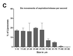
**Fig 3. Size distribution of liposomes as function of aspiration/release speed.** The micrp-emulsions were prepared by 30 aspiration/release cycles of the parasite suspension in a lipid-oil phase using a 1-ml micropipette. (A) one aspiration/release per second; (B) two aspiration/release per second; (C) six aspiration/release per second.
