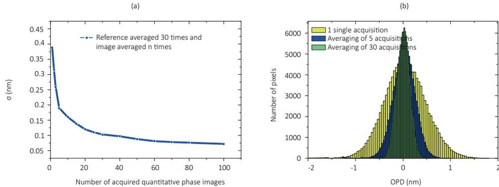
Fig. 7. (a) OPD spatial standard deviation from a sample empty area, versus the number of averaged successive acquisitions. 80 *times* magnification, NA=1.3. Exposure time = 15 ms. (b) OPD histogram evolution with the number of averaged acquisitions.
