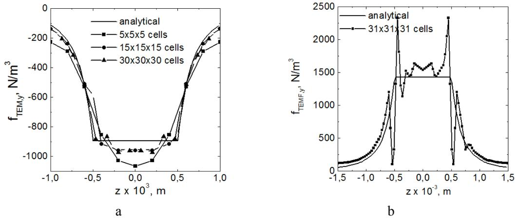
**Figure 4.** Analytical and numerical solutions obtained in a model problem for the y-component of the thermoelectric force along the z-axis, origin of the coordinate system is at the centre of the sphere. The sphere in numerical solution is given with the phase function (15). a.  $S_S - S_L = 1 \cdot 10^{-6} \text{V/K}$  and b:  $S_S - S_L = -1.6 \cdot 10^{-6} \text{V/K}$ , other properties are as in table 1.
