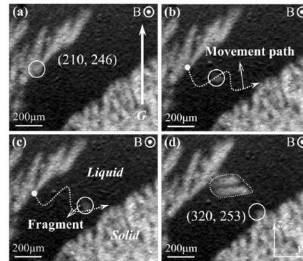
**Figure 2.** Registered detachment of dendrite pieces and their motion in horizontal direction, time interval between the frames (a)-(b) and (b)-(c) is 1.4s. Frame (d) shows detachment of a larger fragment [9].
