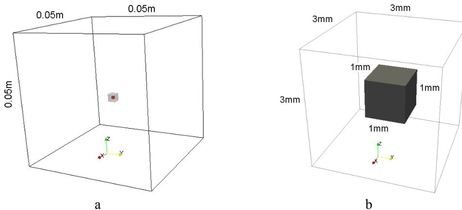
**Figure 3.** Illustration to the domain and sub-domain division in AEQUATIO toolbox. a: complete geometry of the problem with a calculation domain and sub-domain in its centre, particle inside the sub-domain seen as a point and b: sub-domain and the particle
