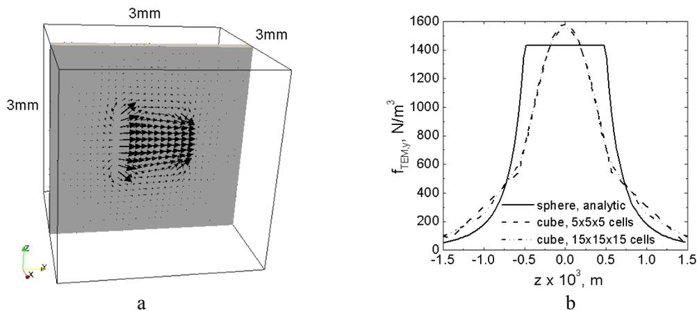
**Figure 5.** Numerical results for a cubic particle  $1\text{mm} \times 1\text{mm} \times 1\text{mm}$  inside the infinite media. a: Vector field of the thermoelectric magnetic force presented in a sub-domain in a plane (yz) which passes through the centre of the particle. b: TEMF distribution along the z-axis with the origin in centre of the particle, analytical solution for a sphere is given as a reference.
