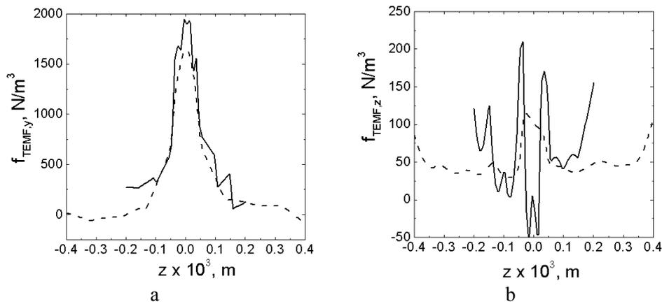
**Figure 6.** Calculated distribution of the y-component (a) and z-component (b) of the TEMF within sub-domains along the z-axis which passes through the centre of each sub-domain, parallel to the thermal gradient. Solid line and dashed lines are for sub-domain  $200\times 400\mu\text{m}\times 400\mu\text{m}$  and  $200\times 800\mu\text{m}\times 800\mu\text{m}$ , respectively. A particle is between  $-0.05\cdot 10^{-3}\text{m}$  and  $0.05\cdot 10^{-3}\text{m}$ .
