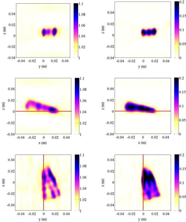
Fig. 2. Reconstructed permittivity map - left: real part and right: imaginary part - at 18 GHz in plane cross-sections. Top: in the  $x = 0$  mm plane, middle: in the  $y = 11$  mm plane, bottom: in the  $z = -7.9$  mm plane.
