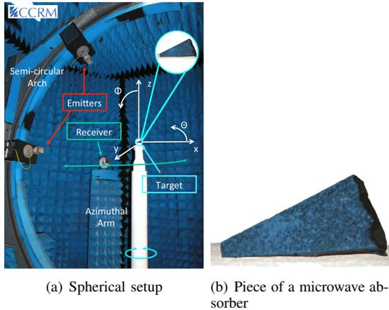
Fig. 1. Pictures of the anechoic chamber setup and of the target
