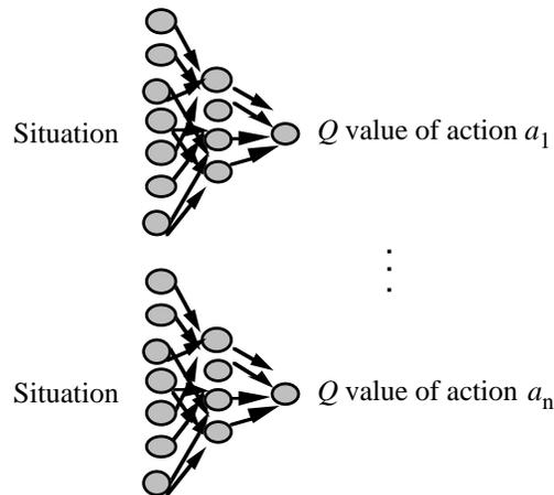
Figure 28. The QCON model: only one output neurone per multilayer neural network. Each network is associated with a unique action and the output is considered as the  $Q$  value associated with the situation-action pair. There are as many QCON networks as there are actions. Generalisation across situation-action pairs is impossible. Learning concerns only one network per iteration.
