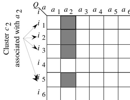
Figure 19. Generalisation using statistical clustering. If one of the situations of the cluster  $c_2$  is the world situation and  $a_2$  as been carried out then all  $Q$  values of the cluster  $c_2$  are updated. In this example, the world situation is  $i_3$  and the action carried out is  $a_2$ , then  $Q(a_2, i_3)$  is updated together with  $Q(a_2, i_1)$ ,  $Q(a_2, i_2)$  and  $Q(a_2, i_5)$ .
