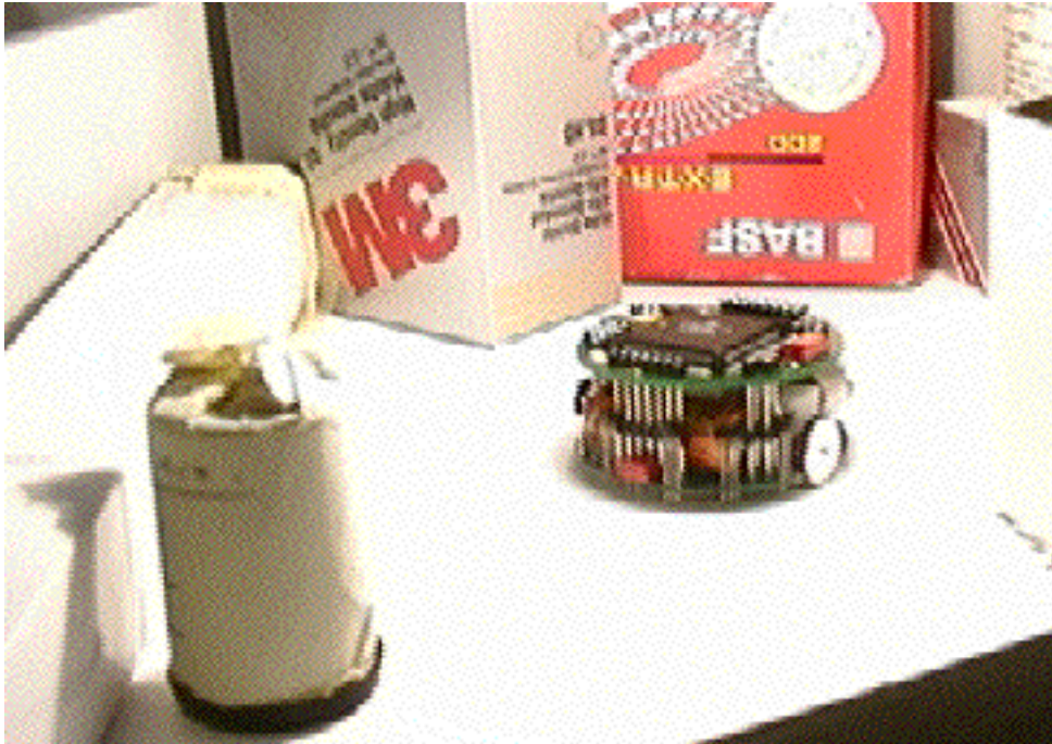
Figure 4. One of the environments of our experiments with the miniature robot Khepera in the centre. Obstacle are put in the arena at the beginning of each experiment.
