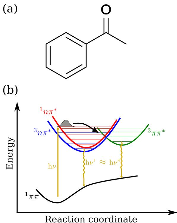
**Fig. 1.** (a) Acetophenone chemical structure; (b) Schematic representation of the  $^1n\pi^*$ -based photochemistry of acetophenone, including  $^3n\pi^*$  and  $^3\pi\pi^*$  triplet populations and eventually phosphorescence.
