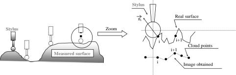
Fig. 11. Measured surface by CMMs
