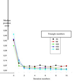
Fig. 9. Median position error according to the number of iterations and the number of triangles.
