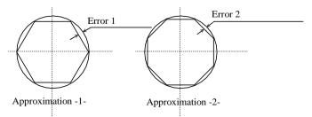
Fig. 7. Approximation errors according to triangle number.
