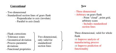
Fig. 12. Comparison between conventional and new approach (Goch et al., 2003).
