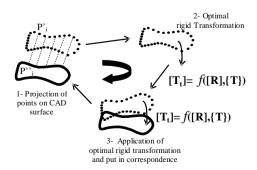
Fig. 3. Principal steps of the I.C.P. algorithm.
