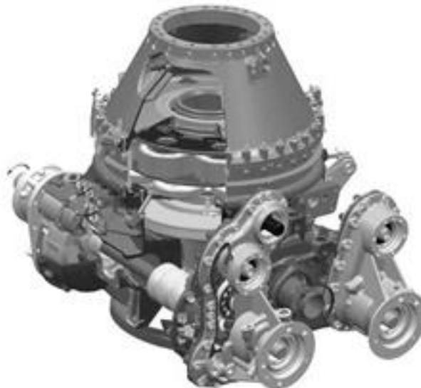
Fig. 1. View of a helicopter main gearbox.
