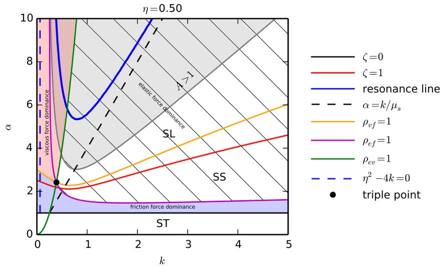
Figure 6: Configuration 4. Map of the block behavior in the  $(k, \alpha)$  plane for  $\eta = 0.5$ . Friction model 1. The light gray area sketches the condition where  $A > 1$ . The friction force is dominant in the light blue area, the viscous dissipation force is dominant in the light red area, and the the hashed area represents the dominance of the elastic force. Also plotted is the triple point where the three forces are of equal magnitude.
