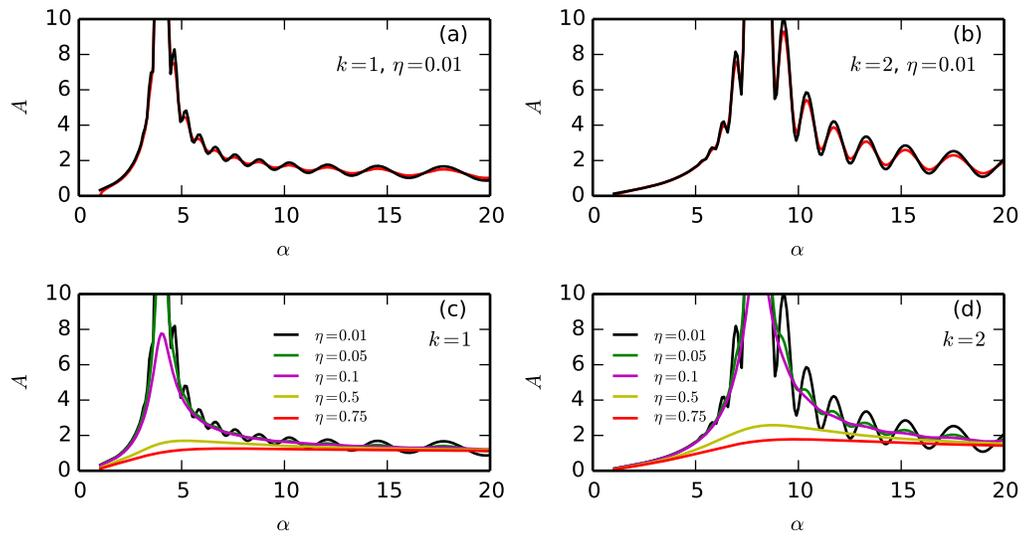
Figure 8: Configuration 4. The block amplitude vs  $\alpha$  for the friction model 1 (red curves) and the friction model 2 (black curves) and for  $k = 1.0, \eta = 0.01$  (a) and  $k = 2.0, \eta = 0.01$  (b). Effect of  $\eta$  for  $k = 1.0$  (c) and  $k = 2.0$  (d) for friction model 1. All curves correspond to an underdamped behavior.
