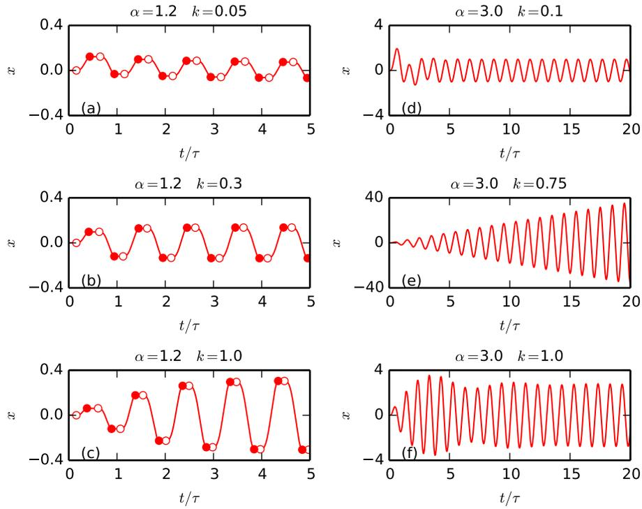
Figure 4: Configuration 3. examples of the motion of the block  $x(t)$  in the stick-slip regime (a, b, c:  $\alpha = 1.2$ ) and in the permanent slip regime (d,e,f:  $\alpha = 3$ ). Curves are computed for the friction model 1. The full symbols indicates a stop of the motion whereas empty symbols indicates a start of the motion.
