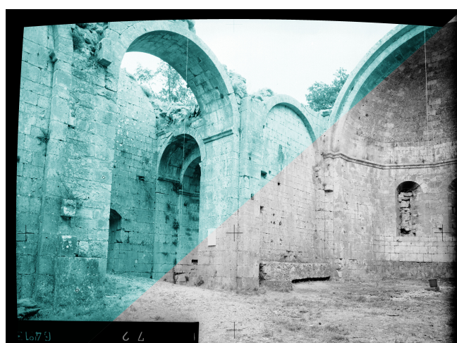
Figure 7. Distortion compensation applied on the pincushion image obtained in Figure 6b. In green the image corrected by inverse distortion; in black and white the original image.
