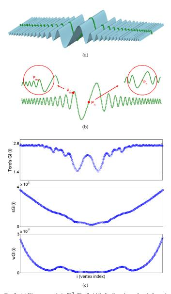
Fig. 2. (a) Wavy rectangle in  ${\rm I\!R}^3$ . The "middle line" on the surface is formed by the vertices lie on the surface with the the same y-coordinate 0.5. (b) The middle line along with zoom on two neighbourhoods around vertices  $P_m$  and  $P_n$ . (c) Values of Toro's GI, sGI and wGI of the vertices located on the middle line.
