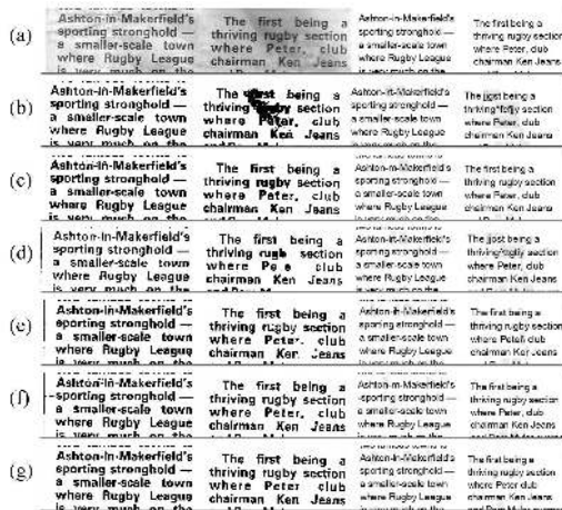
Fig. 14. Document image portion and its corresponding OCR results. (a) Original, (b) Otsu's method [1], (c) Ramirez's method [14], (d) Chen's method [12], (e) Fabrizio's method [16], (f) Sauvola et al. method [4], (g) Proposed method
