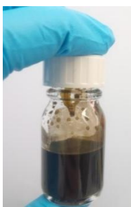
Fig. 9. Famatinite NCs based dispersion
