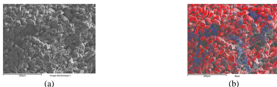
Fig. 1. Analysis of the precipitate formed upon mixing the initial solutions (metal salts in ethanol and sulfur in oleylamine) (a) SEM picture and (b) EDS mapping (sulfur in red, antimony in blue and copper in green)
