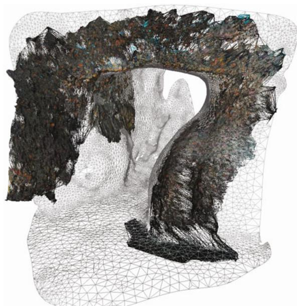
The shots are processed by a synchronous software house, which on one hand trying to calculate beam by adjusting the largest block possible, i.e. the block containing the most triples as possible, then once the block is calculated, the triplets are used to obtain a depth map of the central apparatus producing a dense cloud of 3D point. The adjustment of the beam is therefore only there to ensure the cohesion of these triplets, the 3D points to them being calculated using a single triplet.
