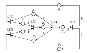
Fig. 2. The TWMG model of an assembly line.
