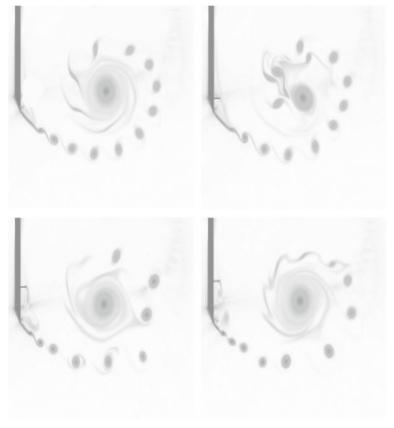
**Fig. 10** Flow past an impulsively started plate with a sharp wedge, angle  $\alpha = 30^{\circ}$  at Re = 9500. Vorticity fields at t = 2.01 for a plate without riblet (*top*, *left*), and for plates with riblets at different positions
