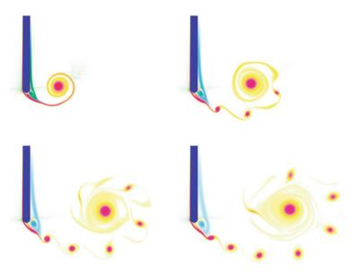
**Fig. 9** Flow past an impulsively started plate with a round edge at Re = 9500. Vorticity at t = 0.39, 0.75, 1.11 and 1.47
