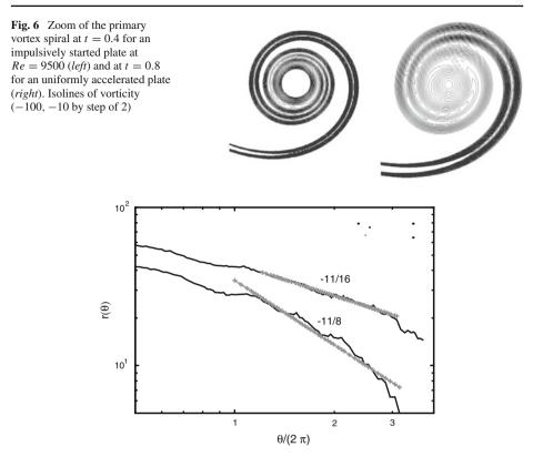
Fig. 7 Scaling of the spiral's radius versus the angle  $\theta$  for both the impulsively started (line with slope -11/16) and for the uniformly accelerated case (line with slope -11/8)
