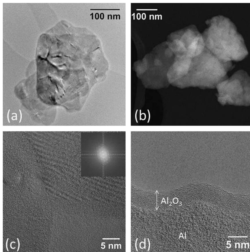
**Fig. 2.** TEM images of the MM-air-16 sample. Platelet morphology is observed (a) and the particles are aggregated (b). The aluminum core is polycrystalline (c) and the amorphous alumina layer has a thickness around  $4.5 \pm 0.5 \text{ nm}$  (d).
