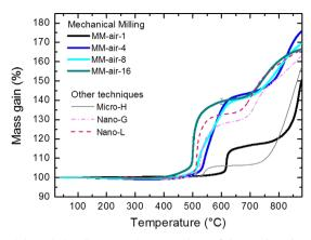
**Fig. 3.** High resolution thermo-gravimetric analyses of the powders obtained by mechanical milling and compared to other elaboration processes.
