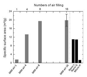
**Fig. 1.** Specific surface area of the powders plotted as a function of the number of air introduction. The results are compared to spherical powders obtained by other elaboration processes.
