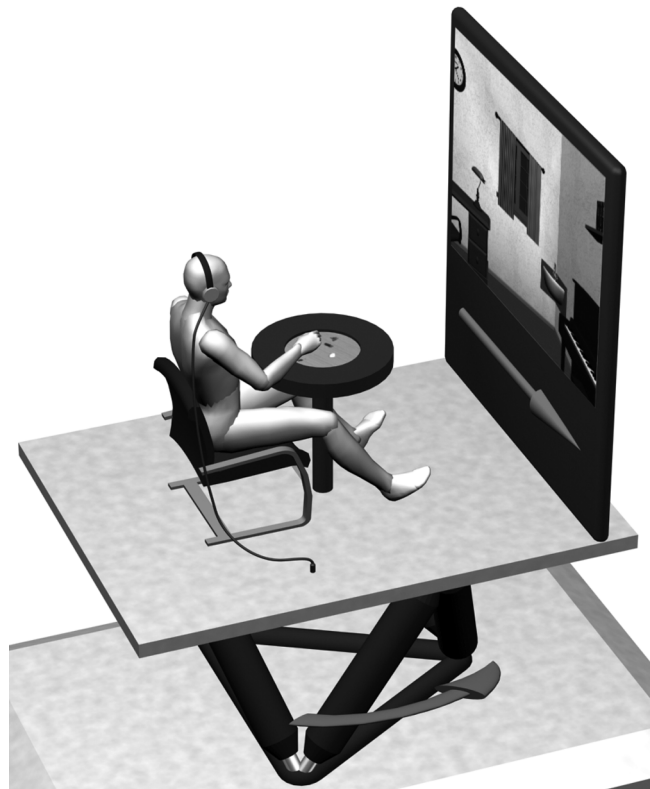
Figure 1. A schematized model of the experimental setup: the moving platform with a front projection screen, a table-embedded screen with a touch-screen, and a noise-cancellation headphone.
