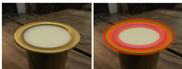
Figure 11: The research area (with dimmed colors) and the extracted arcs of ellipses
