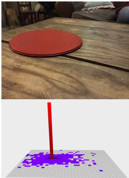
Figure 8: A single ellipse and the Hough Space
