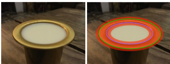
Figure 11: The research area (with dimmed colors) and the extracted arcs of ellipses
