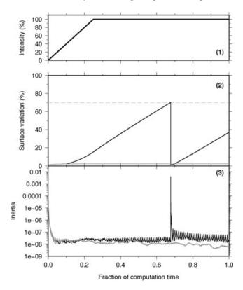
**Figure 4.** Evolution of the inertia ratio criterion, which defines the stability of the computation. Black and grey plots refer to cases with and without erosion, respectively. (1) Progressive introduction of erosion processes. (2) Deformation of the mesh. The ratio between the surface of the most deformed element with respect to the initial surface is plotted. (3) Evolution of inertia during the computation (eq. 8).
