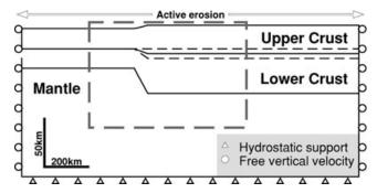
**Figure 3.** Structure of the mechanical model and boundary conditions used in this study. The black dashed lines indicate different depths for the upperlower crust boundary tested in this study. The grey dashed box indicates the location of Fig. 5.
