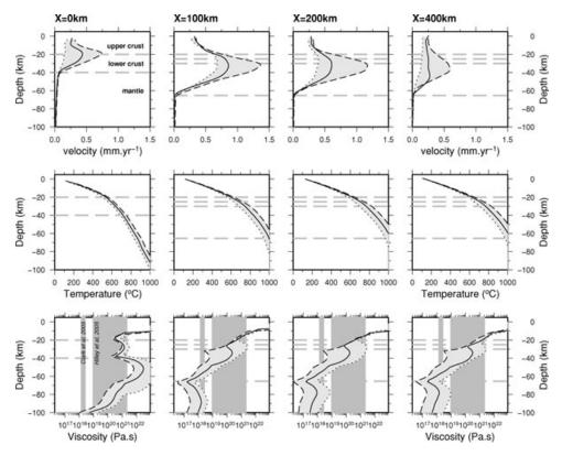
**Figure 7.** Same as Fig. 6. Black solid curves represent the reference model, with erosion, of Fig. 6. The dashed and dotted black curves represent the cases where the limit between the upper and lower crusts is shifted 5 km downward and upward, respectively (Fig. 3). The horizontal dashed lines indicate the positions of that limit (3 depths tested, Fig. 3) and the Moho.
