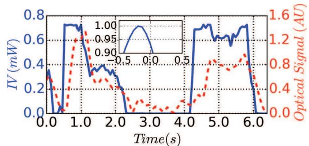
Fig. 3: (Colour online) Temporal evolutions of the electrical power  $IV$  (blue line) and optical signal (red dashed line). The delay is due to the chosen LIA time constant. It can be quantified by the cross-correlation (see inset).
