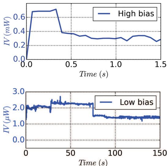
Fig. 2: (Colour online) Temporal evolution of  $IV$ , the electrical power, without feedback. Top: high-bias regime ( $V_{bias} = 1.5$  V,  $G \simeq 3 G_0$  for  $IV \simeq 300 \mu\text{W}$ ). Bottom: low-bias regime ( $V_{bias} = 0.139$  V,  $G \simeq 1 G_0$  for  $IV \simeq 1.5 \mu\text{W}$ ).
