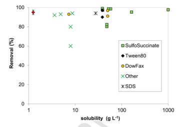
**Fig. 3.** Removal efficiencies compared to the solubility of the pollutant in the considered surfactant (data given in SI, the point form this study is in red with error bars equal to one standard deviation obtained from three replicates). (For interpretation of the references to colour in this figure legend, the reader is referred to the web version of this article.)
