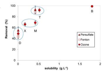
**Fig. 1.** Oxidation removal efficiency related to the solubility of the substance (this study), error bars represent one standard deviation calculated from three replicates and each circle a group of non-statistically different points. Letters show the substance (B: benzene, T: toluene, M: menthol, X: xylene, D: decane).
