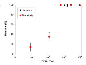
Fig. 5. Removal efficiencies of thermal treatment with vapor pressure of the considered contaminant (data and references given in SI). Errors bars represent one standard deviation
