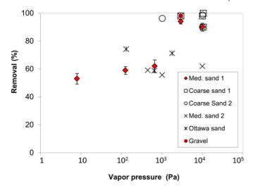
**Fig. 4.** Removal efficiencies during sparging related to the vapor pressure of the compound of interest (results from this study correspond to medium sand 1, other data and references in SI). The points of this study are in red with errors bars that equal one standard deviation obtained from three replicates. (For interpretation of the references to colour in this figure legend, the reader is referred to the web version of this article.)
