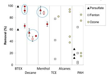
**Fig. 2.** Efficiencies of oxidation differentiated by type of contaminant and oxidant (points measured in this study are in red), error bars represent one standard deviation calculated from three replicates and each circle a group of non-statistically different points. (For interpretation of the references to colour in this figure legend, the reader is referred to the web version of this article.)
