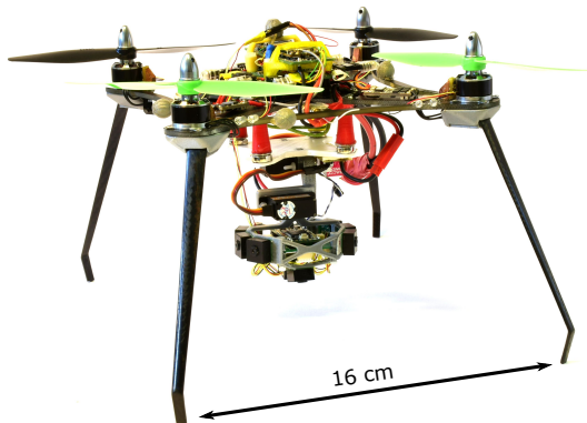
Figure 1: Photograph of the X4-MaG quadrotor with the gimbal case attached below (total mass: 395 g, span: 30 cm, autonomy: 6 min).
