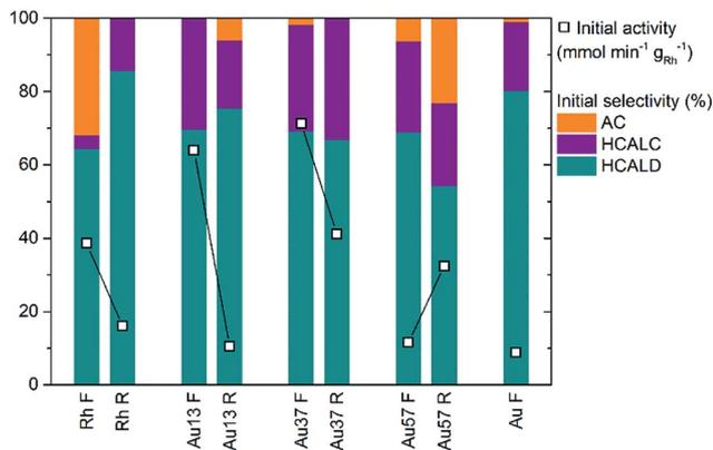
Fig. 8 Initial activities (square dots) and selectivities (bars) in cinnamaldehyde hydrogenation for fresh (F) and pre-reduced (R) AuRh/TiO<sub>2</sub> catalysts. AC, HCALC and HCALD denote hydrocinnamaldehyde diisopropyl acetal, hydrocinnamyl alcohol and hydrocinnamaldehyde, respectively. The initial activity is expressed in mmol min<sup>-1</sup> g<sub>Rh</sub><sup>-1</sup> except for Au/TiO<sub>2</sub> (mmol min<sup>-1</sup> g<sub>Au</sub><sup>-1</sup>). Reaction conditions same as Fig. 7.
