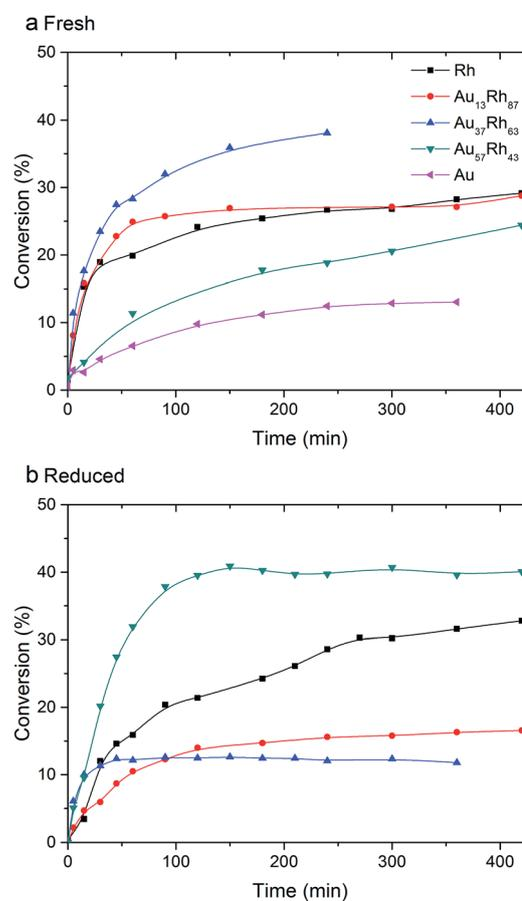
Fig. 7 Evolution of conversions in cinnamaldehyde hydrogenation as a function of the reaction time for fresh (a) and pre-reduced (b) AuRh/TiO<sub>2</sub> catalysts. The reaction was performed at 50 °C under 10 bar H<sub>2</sub> at a stirring speed of 800 rpm.
