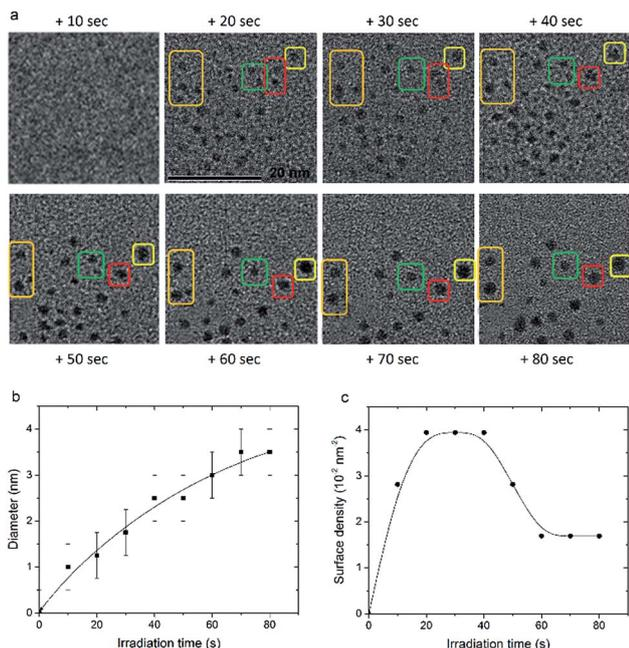
**Fig. 2** (a) *In situ* liquid TEM images showing the nucleation and growth of AuRh nanoalloys in solution during reduction of the precursors by the electron beam. The colored rectangles allow following individual particles. The actual sample size for all images is  $30 \times 30$  nm. The bottom graphs show the corresponding NP diameter (b) and surface density (c) in the solution as a function of electron irradiation time.
