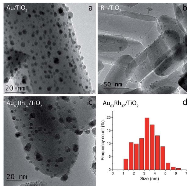
**Fig. 5** Representative TEM images of Au/ $\text{TiO}_2$  (a), Rh/ $\text{TiO}_2$  (b) and  $\text{Au}_{63}\text{Rh}_{37}/\text{TiO}_2$  (c) as-prepared samples. (d) AuRh particle size distribution for the sample depicted in (c).
