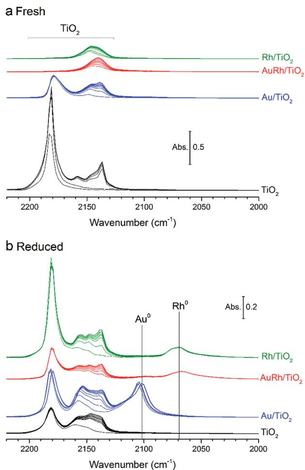
Fig. 6 CO-FTIR spectra of TiO<sub>2</sub>, Au/TiO<sub>2</sub>, Rh/TiO<sub>2</sub> and Au<sub>63</sub>Rh<sub>37</sub>/TiO<sub>2</sub> as-prepared (a) and *in situ* pre-reduced (b) catalysts. The spectra were recorded at increasing CO coverages (2 to 42 μmol CO doses).
