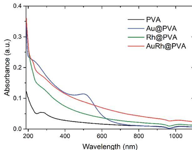
**Fig. 4** UV-vis spectra of the Au, Rh, and AuRh sols stabilized by PVA. For comparison purpose, the UV-vis spectrum of PVA alone is also reported (at the same concentration as that used for sols of metallic NPs).
