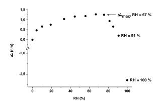
Fig. 3. Evolution of the shift of the LSPR maxima signal vs the relative humidity of the reactor (at room temperature) during the adsorption of water vapor on AEC soot particles deposited on gold nanodisks (+ SiO2 layer).
