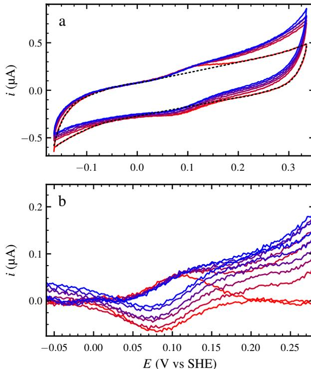
Figure 4: Panels a: raw cyclic voltammograms recorded at increasing concentrations of sulfite: 0 (red trace), 5, 10, 20, 50 and 200  $\mu\text{M}$  (blue trace), together with their baseline (black dashed lines). Panel b: baseline-subtracted data, with the same colors as in panel a. Conditions: : *h*SO immobilized on Au/DTSP/AuNP electrodes, pH 8.4, T = 25°C,  $\nu = 300 \text{ mV/s}$ .
