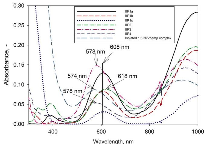
Fig. 3. Reflection UV–vis spectra of IIP1a, IIP1b, IIP1c, IIP2, IIP3, and IIP4 after polymerization and soxhlet-extraction and that of an isolated  $[\text{Ni}(\text{Vbamp})_3](\text{ClO}_4)_2$  complex. Data for IIP4 and the isolated  $[\text{Ni}(\text{Vbamp})_3](\text{ClO}_4)_2$  complex were taken from Lenoble et al. [27].
