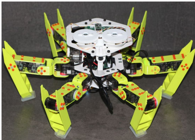
Fig. 1. Top view of the Hexabot robot equipped with the UV-polarized light compass.
