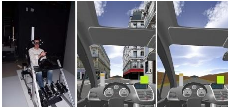
Figure 1: Left: Photograph of participant seated on static driving simulator in operation. Center : screenshot of the first part of the simulated environment (urban scene). Right : Screenshot of the second part of the simulated environment (rural scene).
