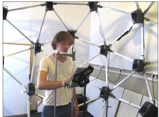
Figure 3. Configuration of the experiment inside the spherical loudspeaker array.
