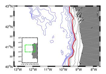
**Figure 1.** Region of calculation of the 3-D FSLE fields. Thick red line: 250 m isobath; Black lines: 50, 100, 150, 200, and 250 m isobaths; Blue lines: isobaths between 500 and 2500 m, drawn every 500 m. Inset: ROMS hindcast region and FSLE region (green rectangle).
