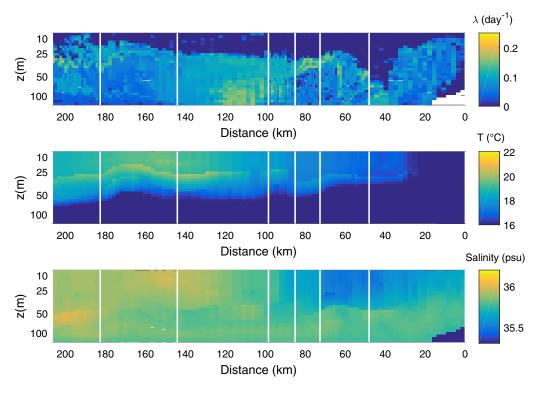
**Figure 6.** Profiles along filament on 26 September 2007. (a) Backward FSLE; (b) Temperature; and (c) Salinity. White vertical lines represent locations of profile of the white circles marked along the profile (white line of Figure 5). Fields were interpolated linearly at 20 equally spaced points in between nodes. Distance along profile increases toward the offshore.
