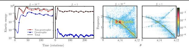
FIG. 3. Left: contributions to the kinetic energy of the flow for two different values of the friction parameter, with  $E=3\times10^{-6}$  and  $512^3$  resolution. Right: corresponding spectral energies processed over the saturated phase. For  $f_r=1$ , the dashed line gives the location of secondary nonresonant interactions of the wave with the base flow  $-2\cos\theta+2\gamma/\Omega$ . The dotted horizontal lines locate the resonance frequency  $\gamma/\Omega$ .
