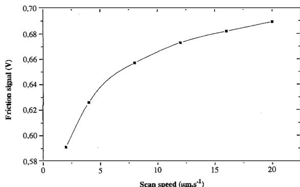
Fig. 11. Evolution of the friction signal for a constant value of  $F_n$  correlated to variation of scan speed during a test on an  $\alpha$ -MoO<sub>3</sub> single crystal.
