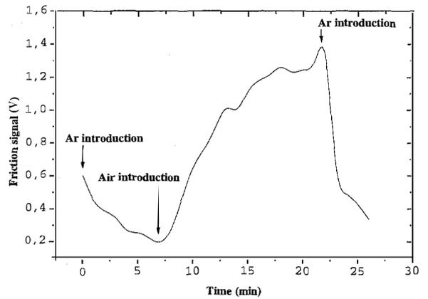
Fig. 10. Evolution of the friction signal for a constant value of  $F_n$  correlated to atmosphere changes during a test on an  $\alpha$ - $\text{MoO}_3$  single crystal. The microscope is set in a proof cell filled alternately with argon and air.
