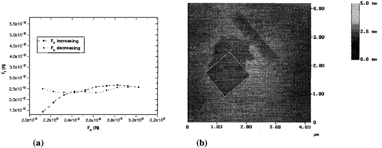
Fig. 4. (a)  $F_f$  vs.  $F_n$  during friction test on a 2H-MoS<sub>2</sub> single crystal. (b) AFM picture recorded after the friction test, exhibiting a depression of the surface.
