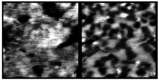
Fig. 4. (a) AFM topographic picture (256 nm  $\times$  256 nm, contact mode, z scale: 2.5 nm) of the sample of Figure 3. (b) AFM friction picture (256 nm  $\times$  256 nm, contact mode, z scale 0.1 V) recorded at the same time. Ordered domains are lightly contrasted in the topographic picture, but appear as low friction areas in the friction picture.
