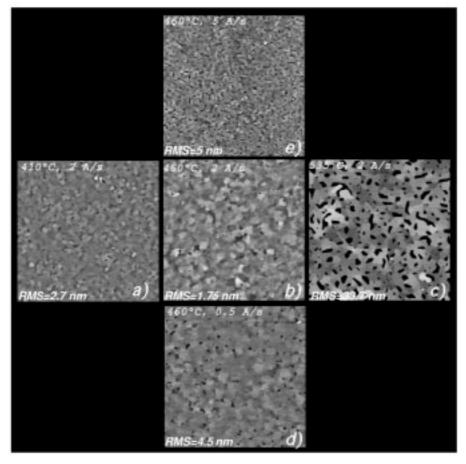
**Fig. 1.** AFM pictures (20.4  $\mu$ m × 20.4  $\mu$ m) of gold films elaborated at three different temperatures: 410 (a, z scale: 10 nm), 460 (b, z scale: 10 nm) and 535 (c, z scale: 75 nm)  $^{\circ}$ C with an evaporation rate of 2 Å s<sup>-1</sup>, and at three different evaporation rates: 0.5 (d, z scale: 20 nm), 2 (b) and 5 (e, z scale: 20 nm) Å s<sup>-1</sup> at 460  $^{\circ}$ C. RMS roughness in nm are given for each sample.
