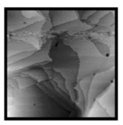
**Fig. 2.** STM picture (500 nm  $\times$  500 nm, bias -1 V, tunnelling current 30 pA, z scale: 5 nm) of a bare gold film elaborated at 460 °C, with an evaporation rate of 2 Å s<sup>-1</sup>.
