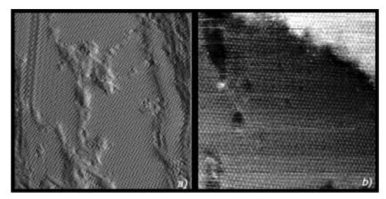
Fig. 7. (a) Current STM picture (50 nm  $\times$  50 nm, bias -1 V, tunnelling current 2 pA, z scale: 2 pa) of a decanethiol film grafted on gold. (b) Topographic STM picture (25 nm  $\times$  25 nm, bias -1 V, tunnelling current 2 pA, z scale: 1 nm) showing the hexagonal compact packing of decanethiol on gold.
