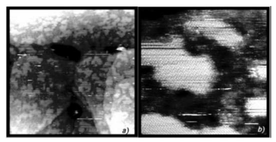
Fig. 3. (a) STM topographic picture (256 nm  $\times$  256 nm, bias -1 V, tunnelling current 2 pA, z scale: 2.5 nm) of a decanethiol film grafted on gold, after 1 s of immersion. The surface is fully covered by the molecules, but exhibit lighter areas which can be attributed in picture b (25 nm  $\times$  25 nm, bias -1 V, tunnelling current 2 pA, z scale: 1 nm) to ordered domains of molecules separated by unordered areas.
