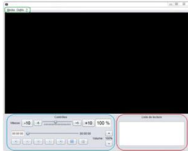
Figure 3 : Graph Interface of Logiral. Black screen: where audiovisual sequences are displayed. Blue outline: control board; contains standard buttons of a multimedia reader, and particularly, the possibility to control the speed of playing by 5% or 10% steps. Red outline: playlist, where audiovisual sequences are stored and ready for playing. Blue and red outlined boxes disappear from the screen after 5 seconds. "Media" menu contains "Read a file," gives access to a file in the computer ready to transfer in the playlist.
