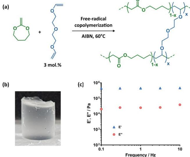
**Figure 5** a) Preparation of degradable bioelastomers by the radical copolymerization of MDO and DIVE. b) Picture of the obtained material. c) Plot of storage  $E'$  and loss  $E''$  moduli as a function of frequency.
