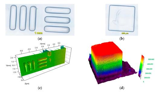
**Figure 6.** Cationic photopolymerization experiments using LED projector @405 nm: (**a**,**b**) patterns (**c**) Profilometry characterization for a thin pattern obtained (thin samples 0.02 mm); (**d**) observation (numerical optical microscopy) of pattern written in 3D for a thicker sample (0.5 mm).
