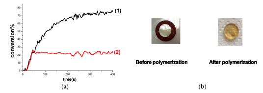
**Figure 5.** (a) Polymerization profiles of TMPTA/EPOX blend (acrylate and epoxy function conversions vs. irradiation time) under air thick sample 1.4 mm upon exposure to LED@405 nm in the presence of Cd7/Iod (0.5%/1% w/w): (1) TMPTA; (2) EPOX; (b) Photos of TMPTA/EPOX film (1.4 mm thick) upon irradiation with the LED@405 nm for 400 s in the presence of Cd7/Iod (0.5%/1% w/w) under air before and after polymerization.
