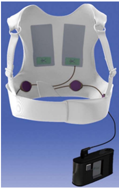
Figure 1 Wearable cardioverter defibrillator. The two defibrillator electrodes are worn on the back of the garment, when the four monitoring electrodes are placed on the elastic belt around the chest. Both systems are connected to the monitor unit.
