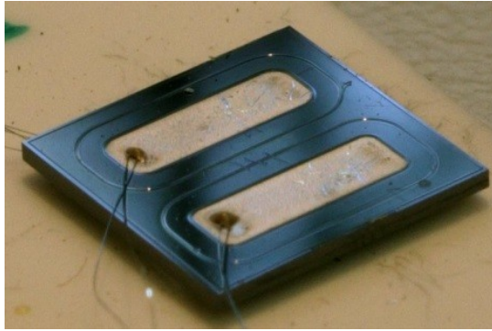
Fig. 4: Typical ISMART SiC diode (here approx. 5 mm × 5 mm) and example of a recorded pulse height spectrum under DT neutron irradiation.
