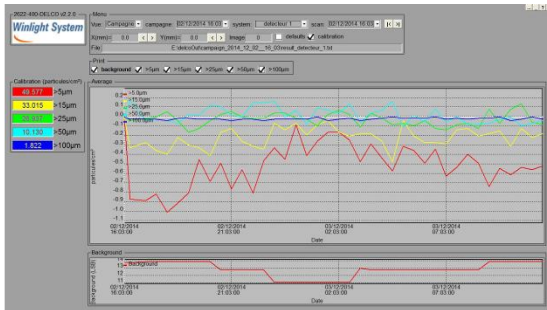
Figure 5. Results for particles counted on the sensor surface of the CLEPART-100 after calibration (ISO 8 cleanroom). x-axis gives the date in days ; y-axis gives the number of particles counted in particles/cm 2 after subtraction of the initial particles present on the glass ( Cf. calibration inset)
