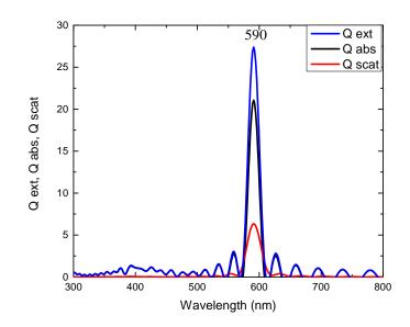
**Fig 2**. (a) Extinction efficiency of a nanoprism in water with different corner radius r, (b) maximum electric field enhancement for r=0 nm and r=4 nm. Radiation is normally incident along z, polarized along x. (c)  $Q_{ext}$ ,  $Q_{abs}$  and  $Q_{scat}$  for r=2 nm.
