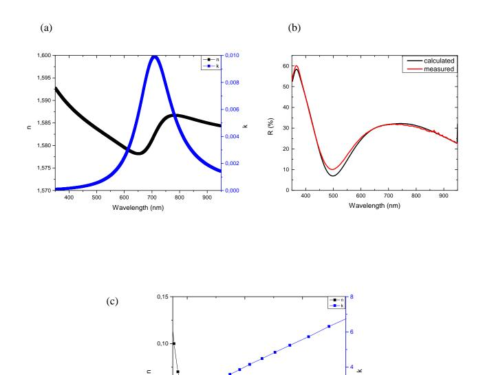
**Fig. 3** (a) Measured n and k of a heterogeneous PVP layer containing in average 25 nm edge size nanoprisms and (b) comparison of measured and by TMM calculated R, (c) n and k for bulk silver from Johnson and Christy<sup>11</sup> for comparison.
