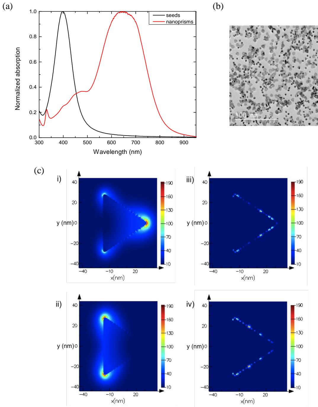
**Figure 1:** a) Normalized absorption of nanospheres and nanoprisms solutions and b) visualization of the electric field enhancement normalized to the incident electric field in the nanoprism for wavelength of peak 1 under z-oriented p-polarized light (i) and s-polarized light (ii) and for the wavelength of peak 2 under p-polarized light (iii) and s-polarized light (iv).
