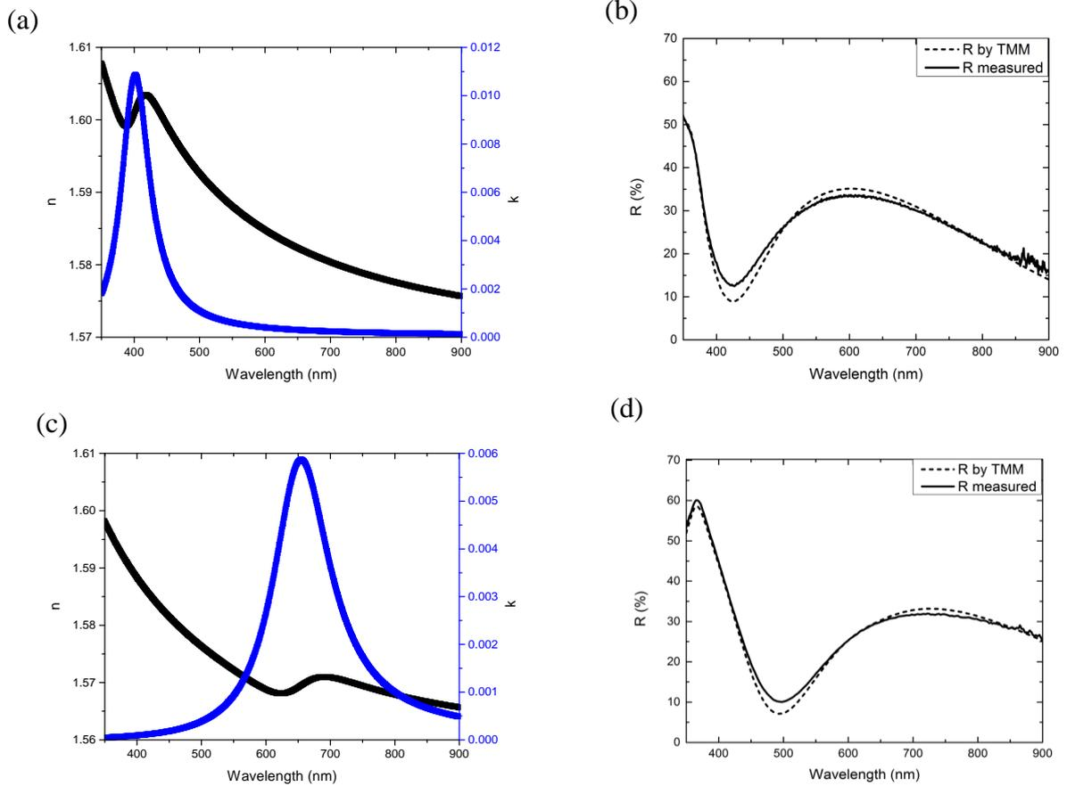
**Figure 3:** (a) Optical indices  $n$  and  $k$  and (b) reflectance measured and calculated by TMM for heterogeneous layers with nanospheres and (c) optical indices and (d) reflectance measured and calculated for heterogeneous layers with nanoprisms.
