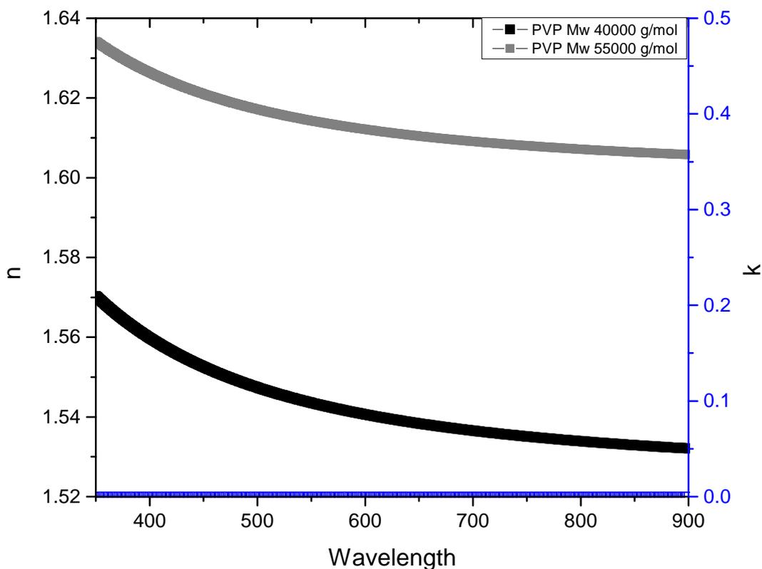
**Figure 2:** Real and imaginary optical indices of PVP of 40,000 and 55,000 g.mol<sup>-1</sup> average molar weight, fitted by a non-absorbing Cauchy law.
