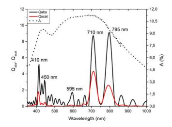
Fig. 5. calculated Qabs and Qscat of the nanosphere-nanoprism system and measured A in PVP.
