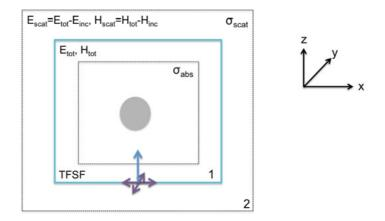
Fig. 1.Cross section of the TFSF source configuration.
