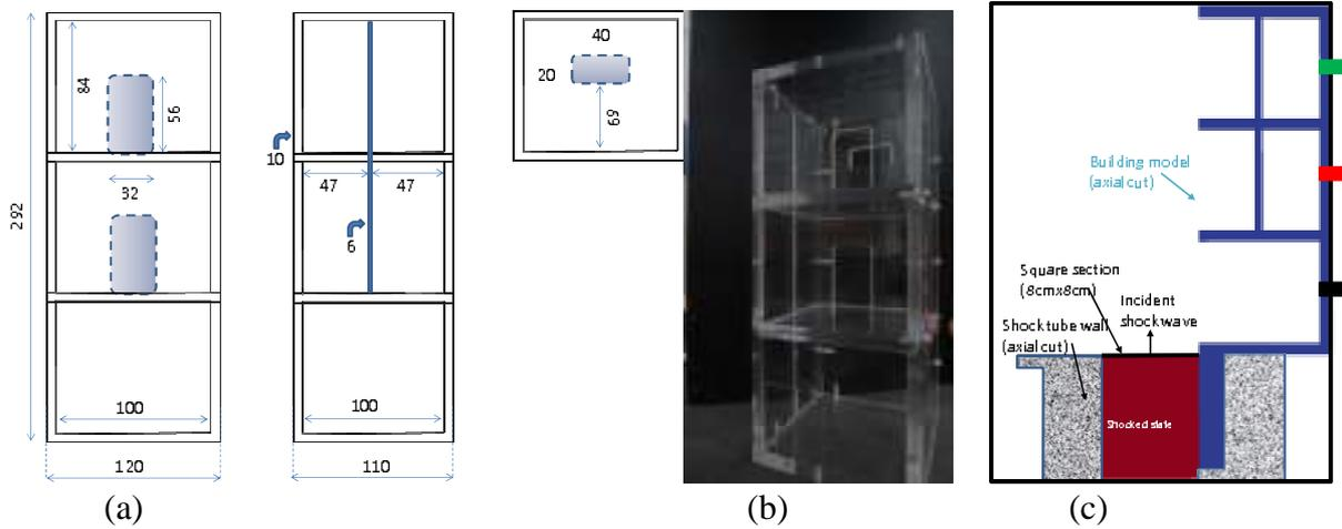
Figure 2: Description and dimensions (in mm) of the tested building model. (a) Schematic drawing of the model; (b) photograph of the Plexiglas building model, and (c) its location (in cm) relative to the shock tube exit.
