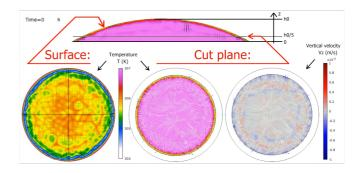
Figure 1 – 3D unsteady computations: thermal and velocity fields over the droplet surface and in a cut plane.
