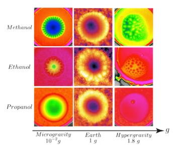
Figure 2 – Top view images from infra-red camera of sessile drop evaporation revealing somehow their internal flow patterns (same thermal conditions but different fluids and gravity levels).
