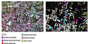
Figure 3: RGB portion of Kaunas image, b) classification by spectral library using full spectral range, c) classification by spectral library using selected bands, and d) classification by spectral library using selected bands, and regularization step.
