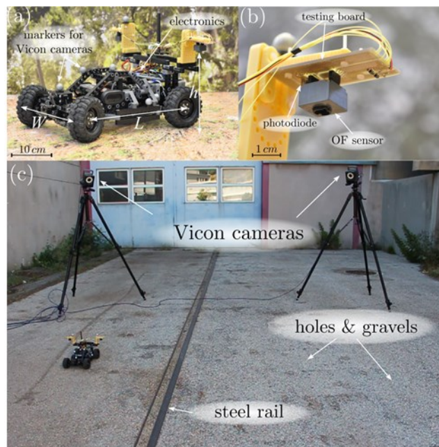
Fig. 1. (a) The low-cost car-like robot called BioCarBot. (b) One of the two OF sensors used on the robot. (c) The outdoor test environment equipped with Vicon cameras. The ground, which consisted mainly of asphalt, included holes, gravel and a disturbing steel rail. Adapted from [13].
